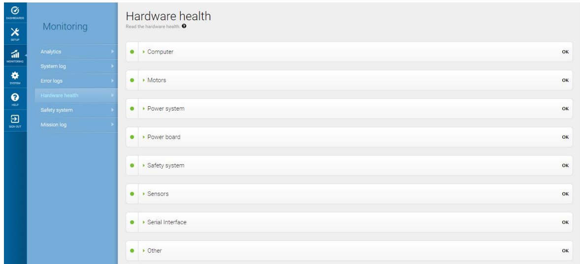
Figure 19.1. The interface in Hardware health displays which component is failing and often for what reason.
