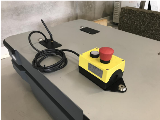
Figure 10.1. MiR250 has one Emergency stop button that must be connected through the electrical interface. You can also connect the interface to a series of additional Emergency stop buttons.
