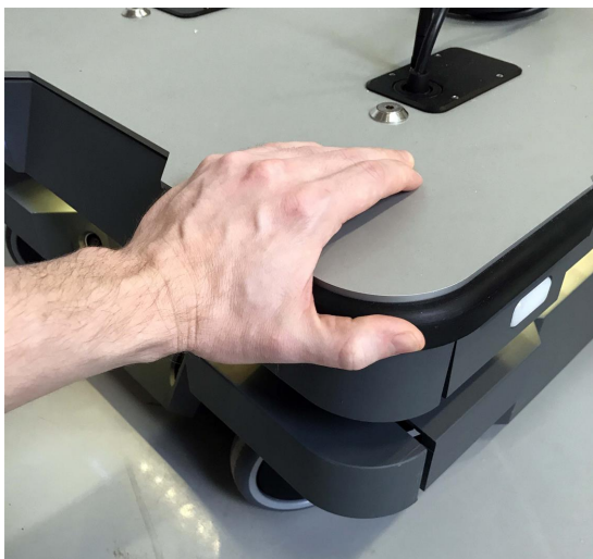
Figure 6.3. When pushing the robot, only push on the top plate.
