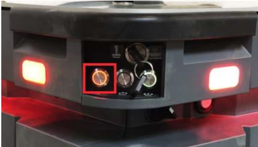
Figure 10.2. The Stop button is the left-most button on the control panel.
