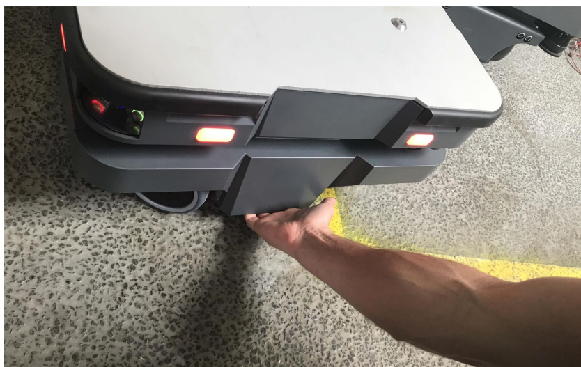
Figure 6.4. When pulling the robot, use either the front pull handle or the rear pull handle.
